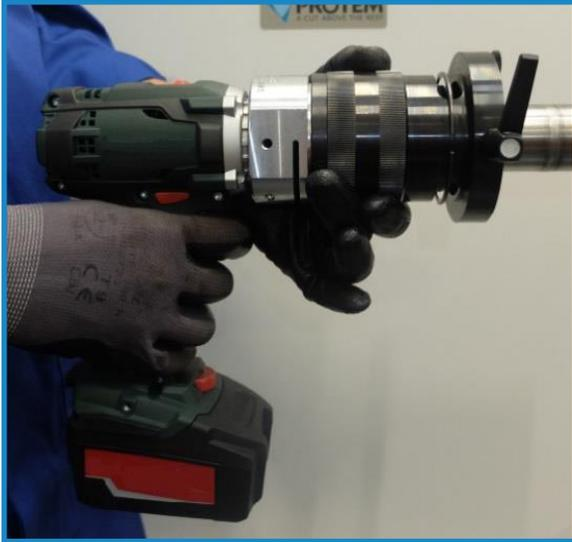
The OD Mounted Facing machine SE25 clamps on the outside  $\varnothing$  of the tube with clamping collets. One collet per  $\varnothing$  is necessary.
