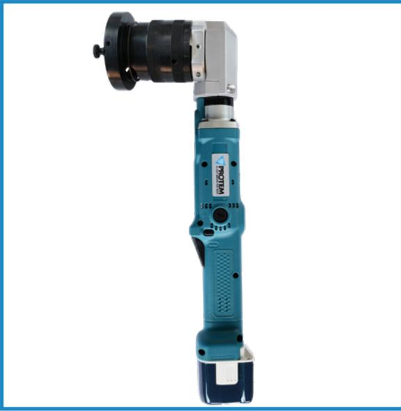
The OD Mounted Facing machine SE65RA clamps on the outside  $\varnothing$  of the tube with clamping collets. One collet per  $\varnothing$  is necessary. No distortion of the tubes, even for the thinnest ones.
