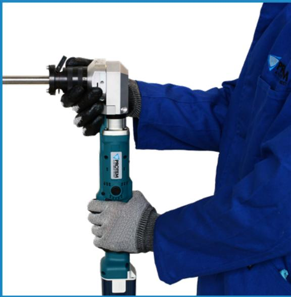
The OD Mounted Facing machine SE25RA clamps on the outside  $\varnothing$  of the tube with clamping collets. One collet per  $\varnothing$  is necessary. No distortion of the tubes, even for the thinnest ones.
