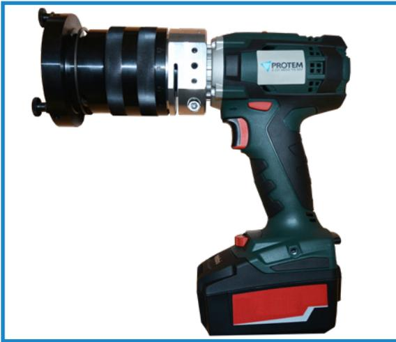
The OD Mounted Facing machine SE65 clamps on the outside  $\varnothing$  of the tube with clamping collets. One collet per  $\varnothing$  is necessary. No distortion of the tubes, even for the thinnest ones.
